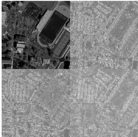
Figure.1. LL, LH, HL, and HH subbands of a satellite image obtained by using DWT.
